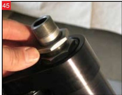
45 Install the second nut (jam nut) onto the lower nut.
