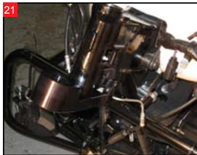
The bottom adaptor is in place.
