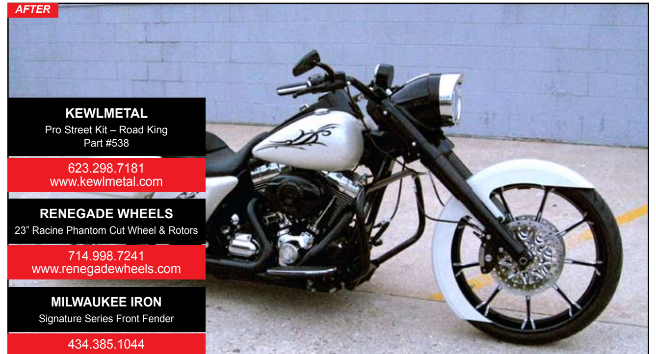
That's 45 degrees of neck rake you're looking at, and no torch was used. Want one for your bike? Contact Kewl-Metal and tell them American Bagger sent ya.
