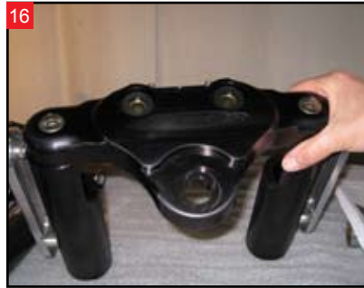
The top triple clamp has the spacer tubes attached. They must be removed.
