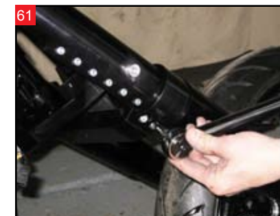
61 Tighten the lower triple clamp pinch bolts on both sides.
