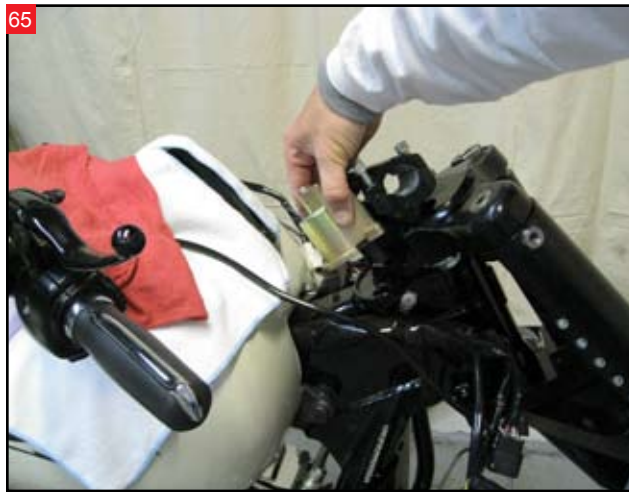
Install the ignition switch bracket.
