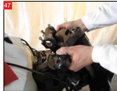
47 Install the top triple clamp with all the components already installed.
