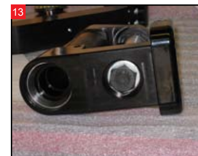
This is the adapter block bolt.
