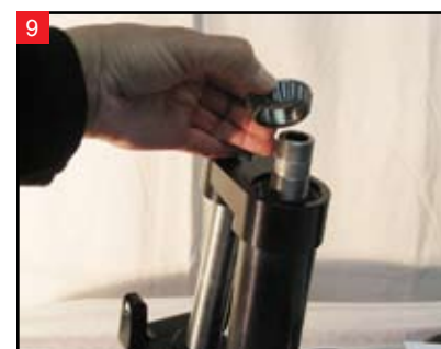
Remove the upper bearing.
