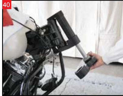
40 Slide the lower triple clamp and fork stem assembly into the adaptor assembly.
