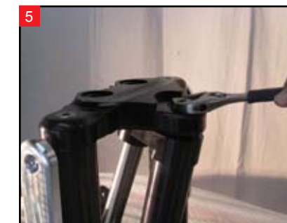
Loosen the top nut on the KewlMetal triple clamp assembly.
