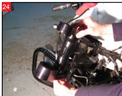
Engage the threads in the top adaptor block and hand tighten.
