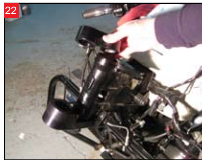
Set the top adaptor plate into place.
