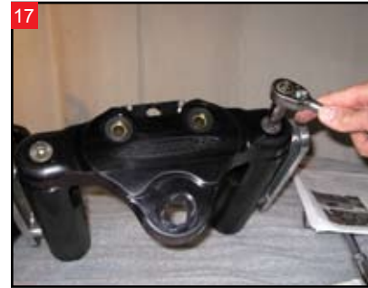
Loosen the bolts that hold the spacer tubes in the top triple clamp.
