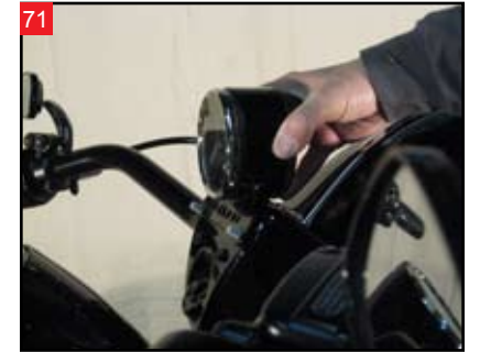
Install the instrument module and ignition switch.
