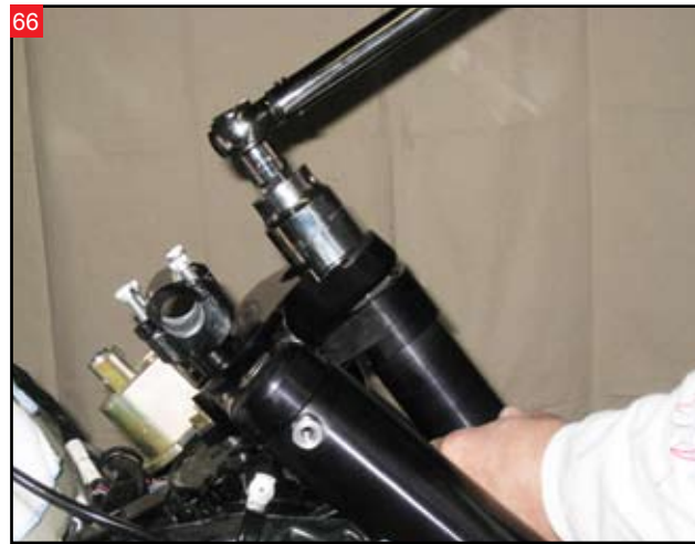
Tighten the fork stem nut.
