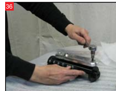
Dismount the covers from the Pinching Fat Fork Tubes.
