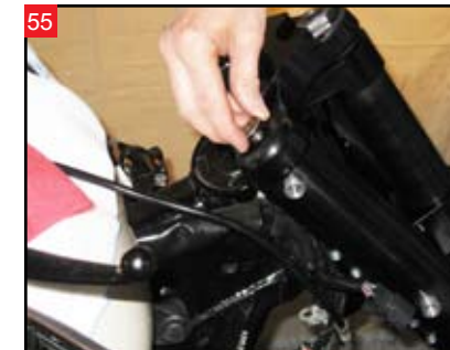
55 Engage the threads of the tube assembly on each fork tube with the upper tube bolt.
