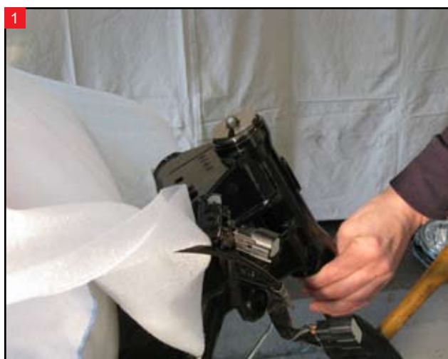
The existing inner neck bearing races (top and bottom) need to be popped out of the neck. A couple of whacks usually breaks them loose.
