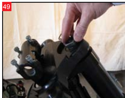
49 Install the stem nut onto the stem.
