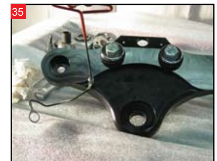
Attach the ground wire removed from the stock triple clamps.
