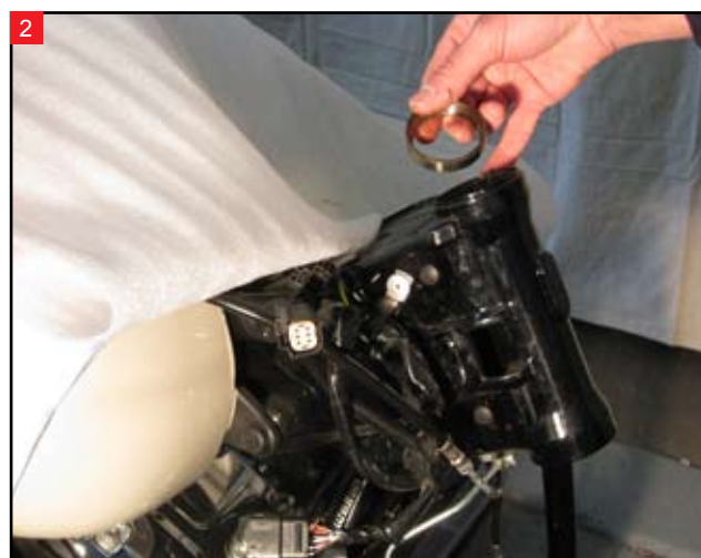
Remove the upper bearing race.
