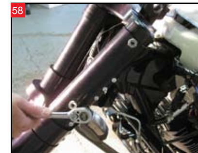
58 Tighten the pinch bolts.
