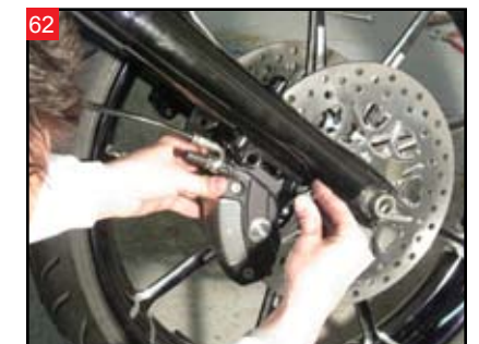
62 Install the front brake calipers.
