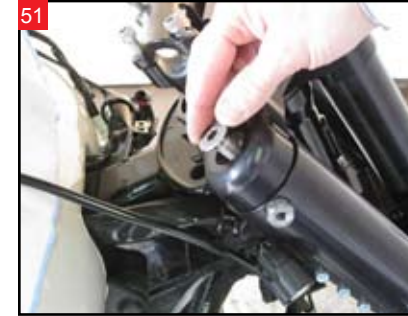
51 Thread the Pinching Fat Tube bolts into the tubes through the triple clamp, but leave them loose.
