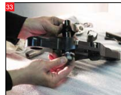
Install the lower riser halves into the triple clamp.
