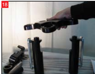
Separate the spacer tubes from the triple clamp.
