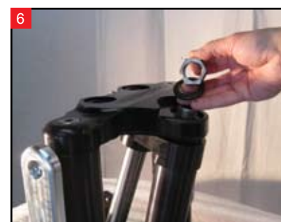
Pull the nut and washer off the stem.
