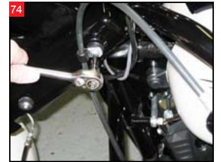
Attach the clutch cable loom, then go back and check/tighten all the hardware.
