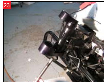
Slide the grade 8, 3/4" x 10" hex-head bolt up through the two adaptor plates.
