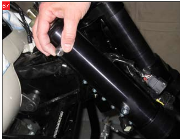
Install the fairing mount hardware.
