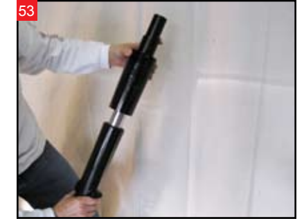
53 Slide a lower Fat Fork Cover onto each tube with extension in place.
