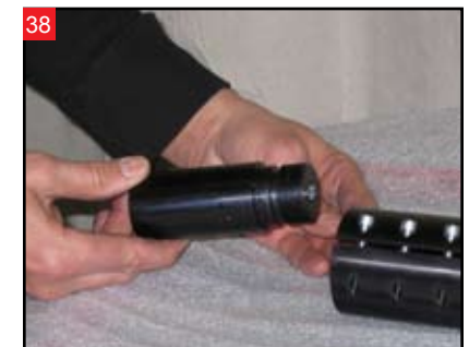
Remove the fork extension cap.
