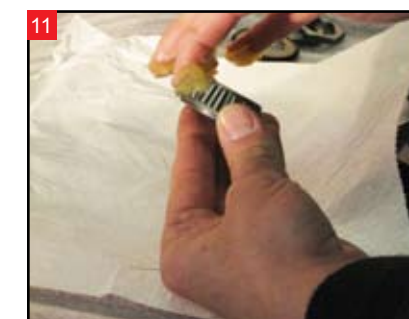
Thoroughly grease the upper bearing.
