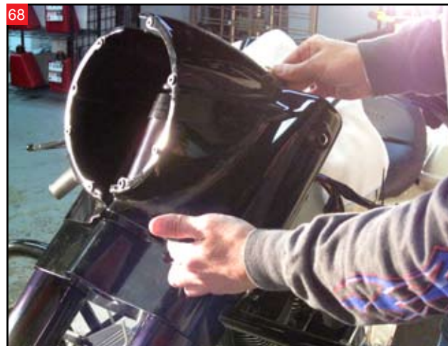
Install the lower shroud and headlight cowl.
