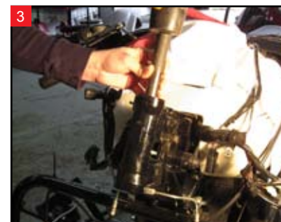
Now tap the bottom inner bearing race loose.
