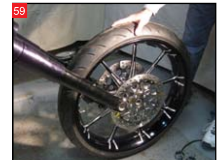
59 Install the front wheel/tire assembly.
