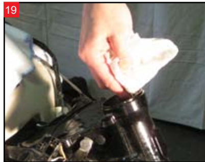
Clean the bearing races in the neck.
