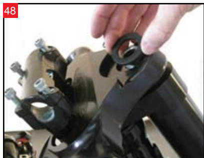
48 Install the large washer on the stem.
