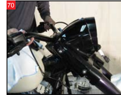
Install the handlebars and riser cover.
