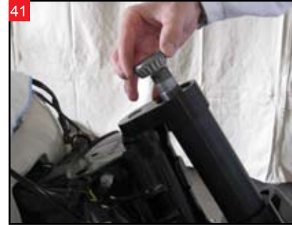
41 Slide the upper bearing onto the fork stem.
