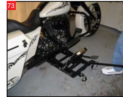
Lower the bike down to the floor.
