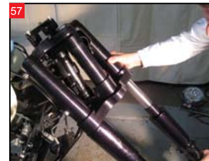
57 Slide the other fork tube into the triple clamps.
