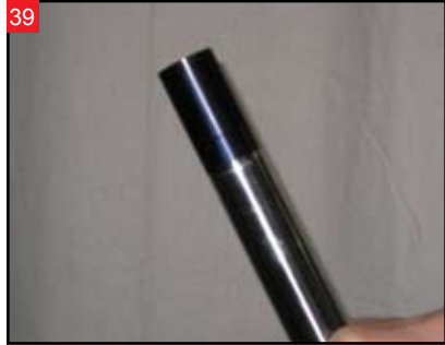
39 Install a fork extension cap onto each fork leg top.
