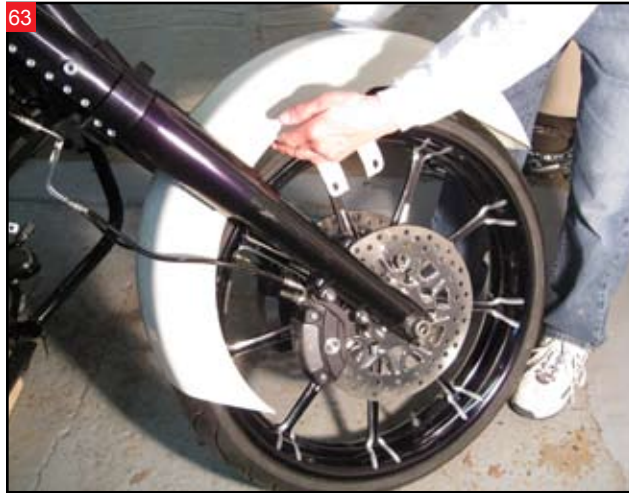
Install the front fender.
