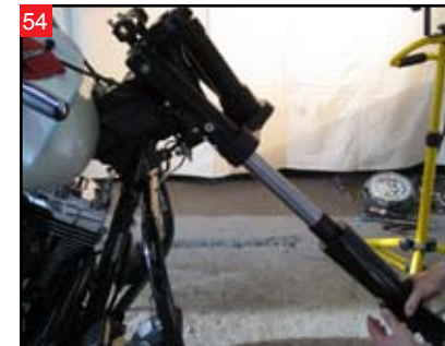
54 Slide the fork tube assemblies into the triple clamps.
