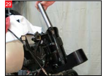
Install the inner spacer tube.
