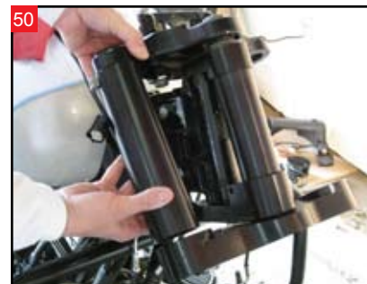
50 Install the Pinching Fat Fork Tubes between the upper and lower triple clamps.
