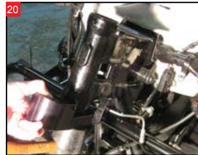
Install the bottom adaptor block by tapping it into place.
