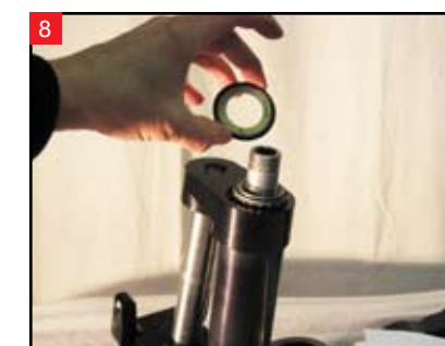
Pull the bearing seal off of the stem.
