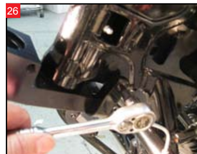
Install and tighten the two bolts in the neck (one on each side).
