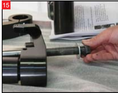
Pull the bolt out.
