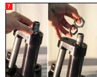
Now pull the two lower nuts off of the KewlMetal stem.
