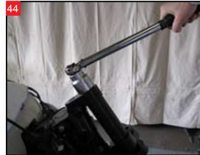
44 Tighten it down against the bearing.
