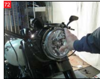
Install the headlight and headlight rings.
