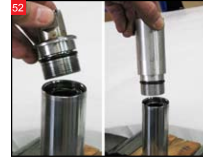
52 Remove fork caps from the tube assemblies and transfer cap seal to the tube extension, then thread extension into place in each tube.
