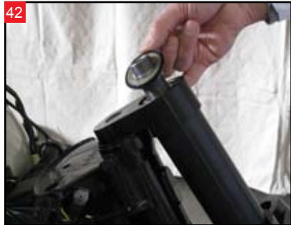
42 Install the dust seal over the stem on top of the bearing.
