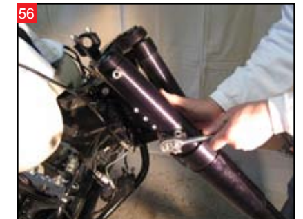
56 Tighten the pinch bolts.
